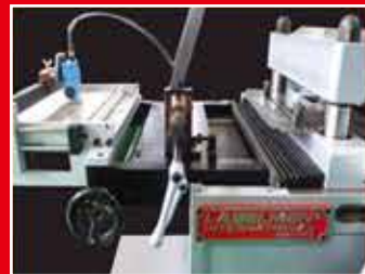
可移動式護膜裝置 ADJUSTABLE LAMINATING DEVICE
