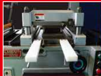
可替換式沖壓/模切座 REPLACEABLE PUNCHING/ DIE-CUTTING STATION
