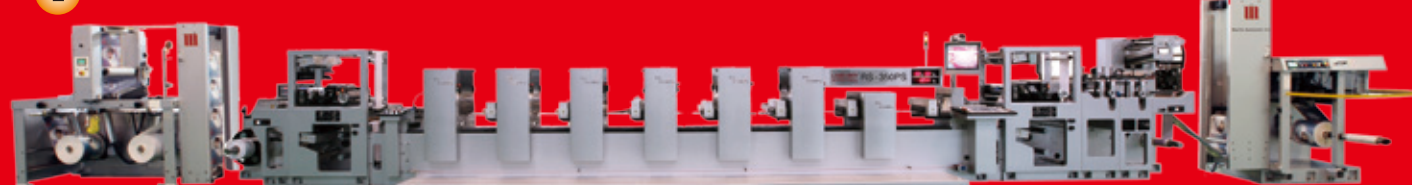
RS-350PS 6-Color Full Rotary/Intermittent Offset Printing Machine
