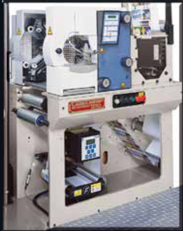
輪轉式網版印刷座 STORK ROTARY SILK SCREEN PRINTING STATION
