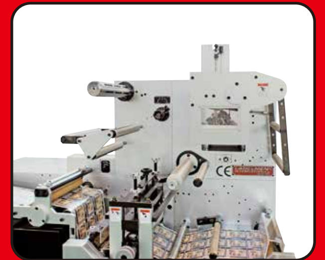
不停機排廢系統 NON-STOP WASTE REMOVAL SYSTEM
